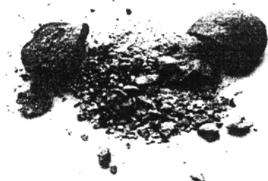
Fig. 3. Limestone specimen after tests. q = 0.5 \cdot 10^4 \text{ kW/m}^2 .
